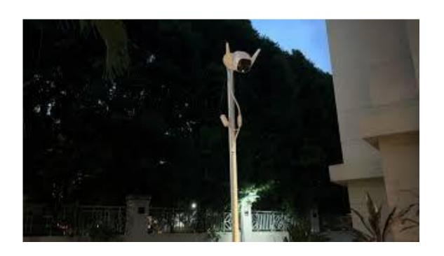
A self contained kit for mobile deployments that includes a HUB, 4G LTE internet, a PTZ camera, a battery and an industrial socket point for charging, all packaged in an IP66 weatherproof enclosure.
